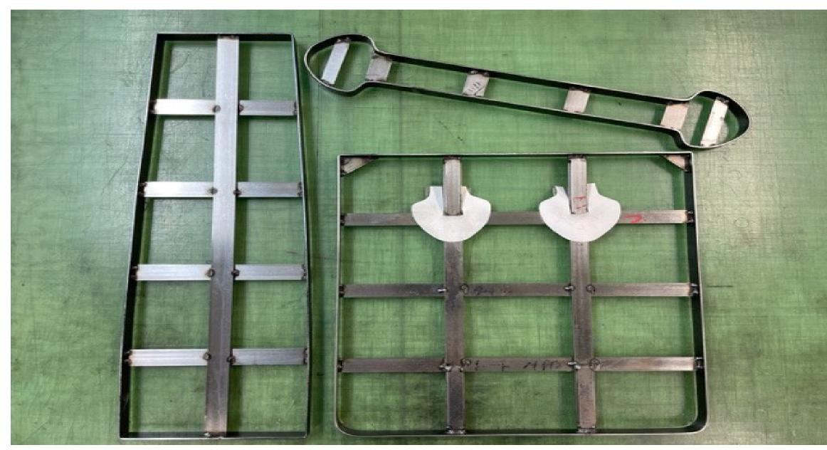
Conventional cutting dyes(3 sets of blade) for ONLY 1 type of temporary hand bag manufacturing
